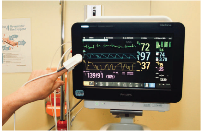
Phillips Monitor and Pulse Oximeter which fits on the finger for measuring oxygen saturations
